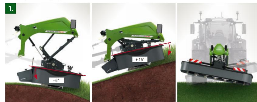
Transverse pendulum angle of +/- 13°
