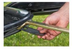
The quick-change system with practical special tool makes changing the knives foolproof.
