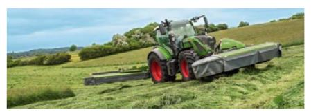
The generous ground clearance enables quick and safe turning on headlands, and the compensating cylinder on the outrigger keeps the mower stable on headlands.
