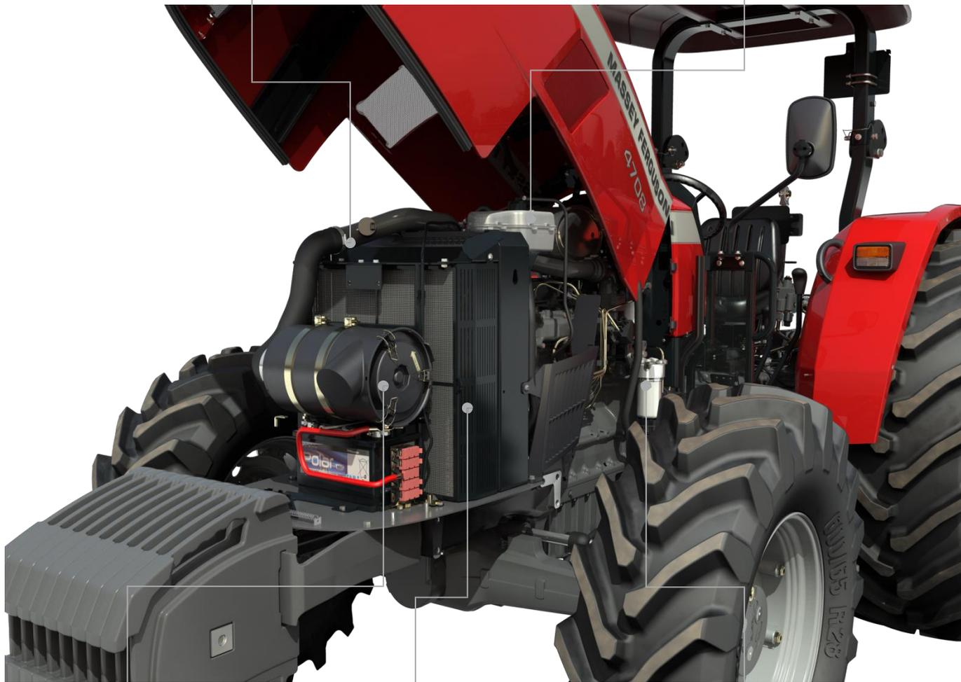
Dry element air filter is fitted for simple and effective filtration
