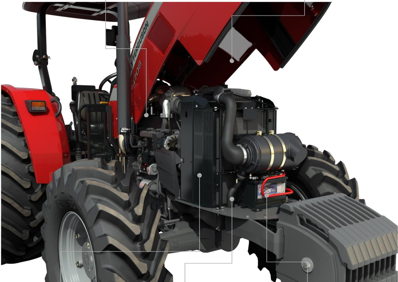
Easy to clean cooling package including fuel cooler and engine radiator
