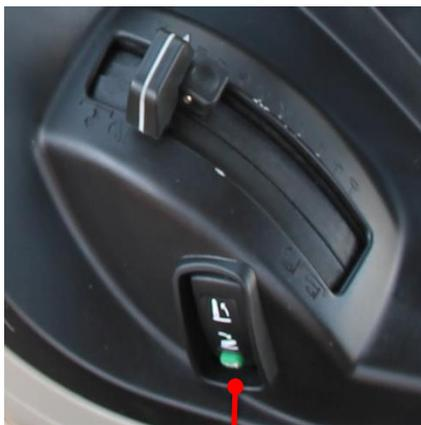
**Up/Down rocker switch with quick soil engagement**
