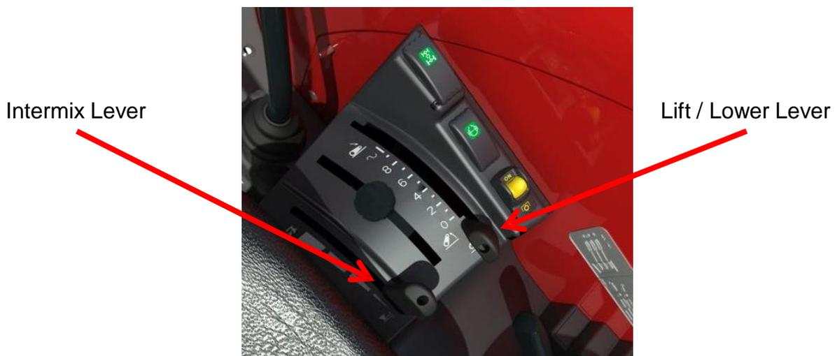
ELC with position / intermix / draft control for enhanced productivity with linkage mounted implements.
