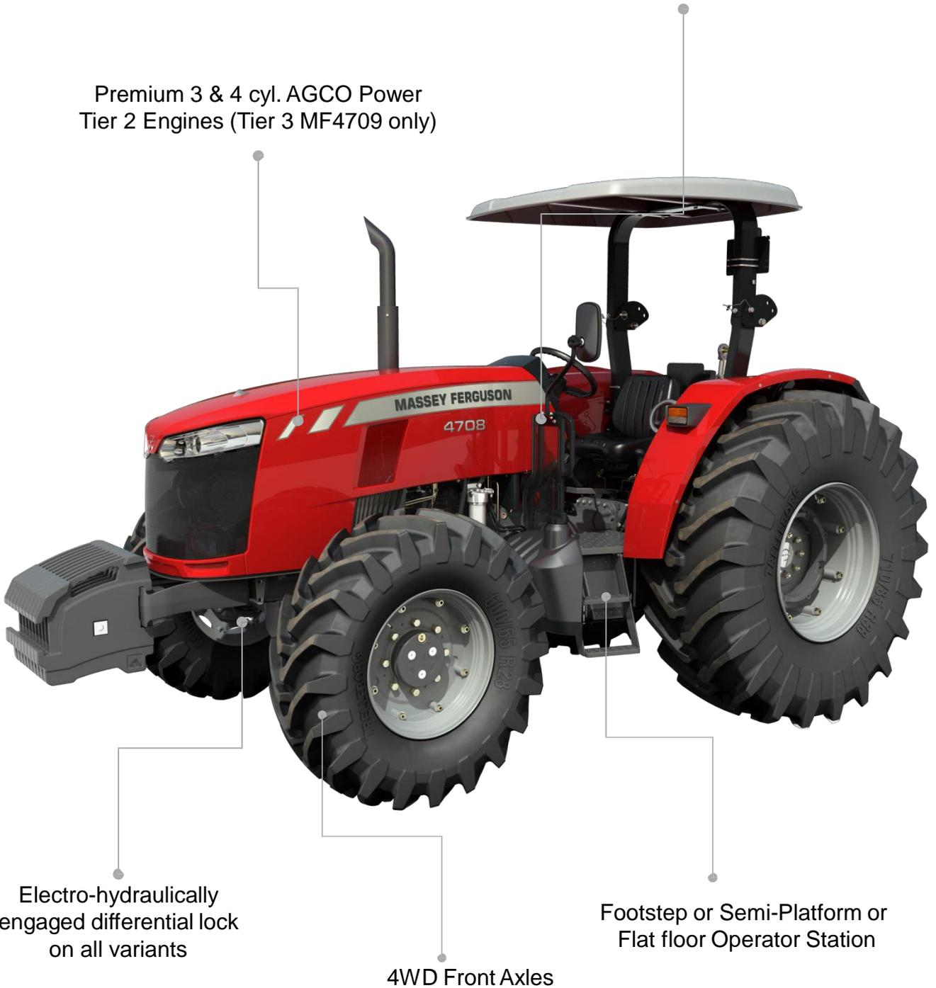
Electro-hydraulically engaged differential lock on all variants
