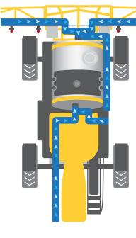
Rain, wind and a hundred other things can stop a job before it's done, letting residues settle in the plumbing. ClearFlow<sup>™</sup>, the industry's first full-recovery system, pushes unused product from the plumbing back into the tank, prior to a tank or boom rinse. Product goes back in the tank to be reagitated or off-loaded, minimising waste and contamination. So you'll be confident plumbing and booms are clean.
