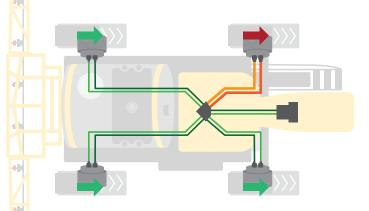
SmartDrive, standard on every machine, continuously and independently controls each wheel, so each wheel always gets all the torque it needs, when it needs it. Wheel slip is automatically countered by sending more power to the gripping wheels, while managing the slipping wheel to regain traction. The best part: you don't even have to tell it to do it. **EASY TO OPERATE & CREATURE COMFORTS**
