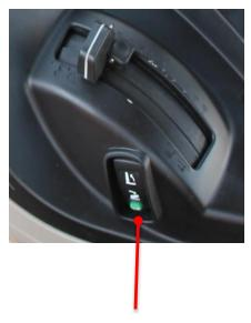
Up/Down rocker switch with quick soil engagement
